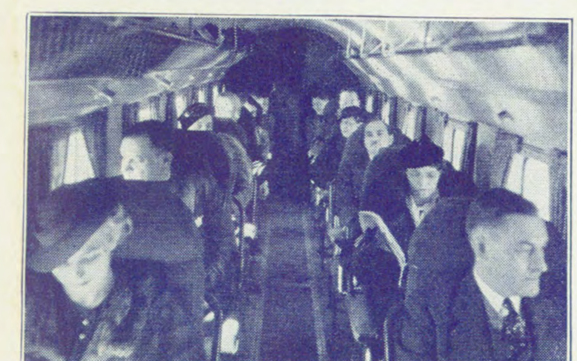
Thermostats control steam heat in Douglas cabins. Chairs reverse or recline to any degree.
