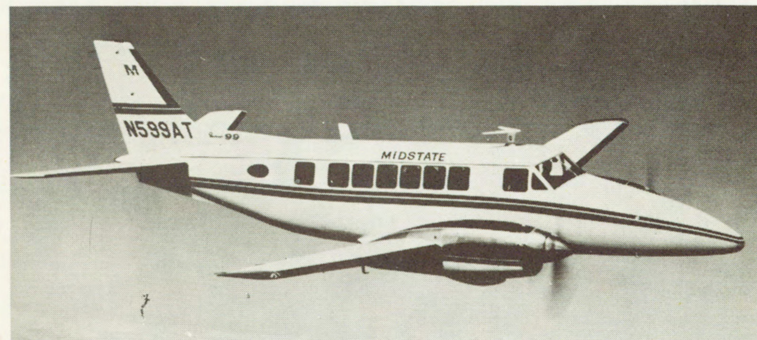
B99 Beechcraft 15-passenger twin-engine Jet prop aircraft.
